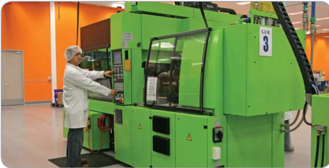
Injected moulding machine.
